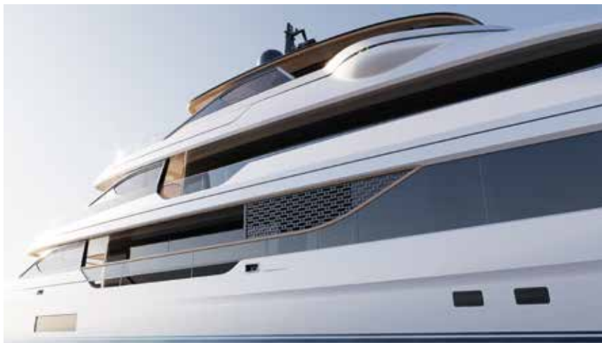
These pages: Panorama 50 created in collaboration with the Piredda & Partners studio. It is a 50-metre steel yacht with aluminium superstructure. It features select, natural materials like light wood, stone and rough metals, and has a panoramic owner's cabin on the forward upper deck. This first unit marks Admiral's entry into series production
